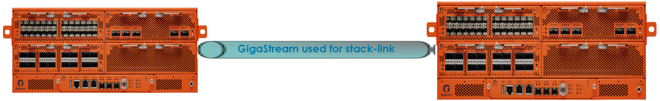
Figure 62: Daisy-Chain Configuration using GigaStream for Stack-link
